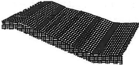
ON SHALLOW SLOPES, STRIPS OF PROTECTIVE COVERINGS MAY BE APPLIED PARALLEL TO DIRECTION OF FLOW.
