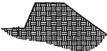
WHERE THERE IS A BERM AT THE TOP OF THE SLOPE, BRING THE MATERIAL OVER THE BERM AND ANCHOR IT BEHIND THE BERM.
