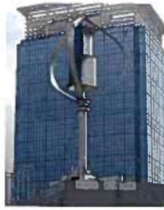
**Figure 5: Vertical Axis Turbine** <sup>6</sup>
