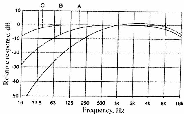
Figure 3. Definition of A, B, and C Frequency Weighing Scales (Beranek and Ver, 1992)
