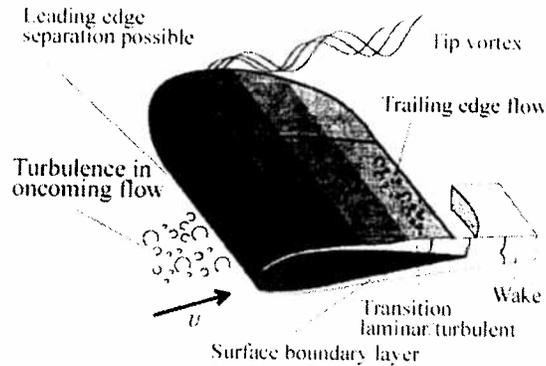
Figure 6. Schematic of Flow Around a Rotor Blade
