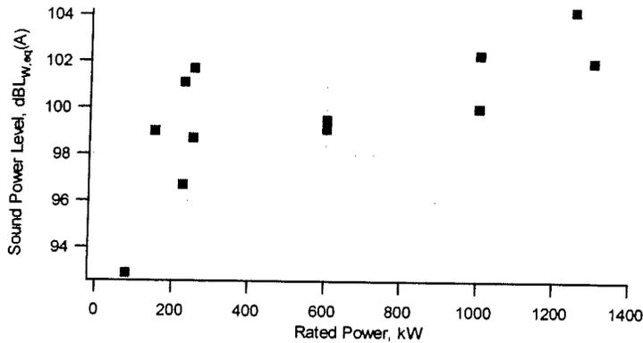
Figure 9. Sample measured wind turbine sound power levels
