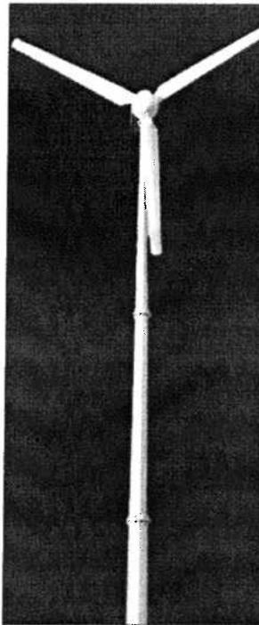
The Hummer 20kW wind turbine is a low wind speed, direct drive generator.
